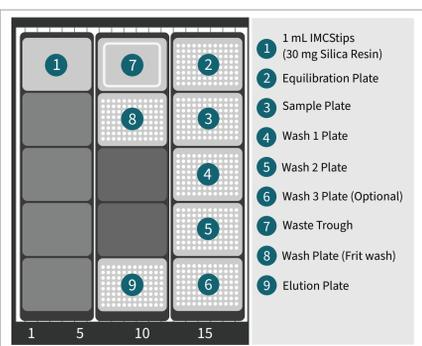
Figure 3. Deck layout of the automated plasmid purification on a Hamilton ML STAR.
