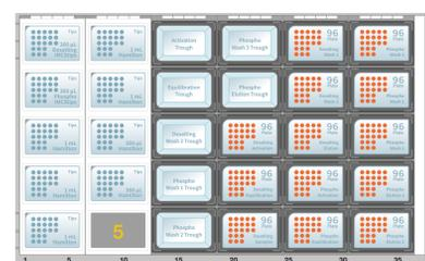
**Figure 5.** MicroSTAR deck layout for the automated method for desalting and phosphopeptide enrichment.
