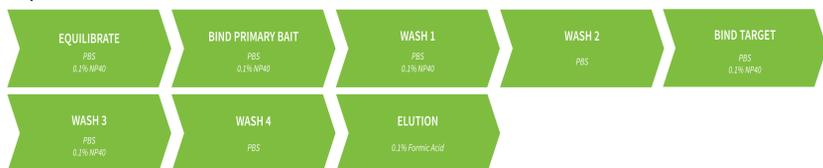
Table I. INTip chemistry workflow using MabSelect SuRe LX 50 µL resin
