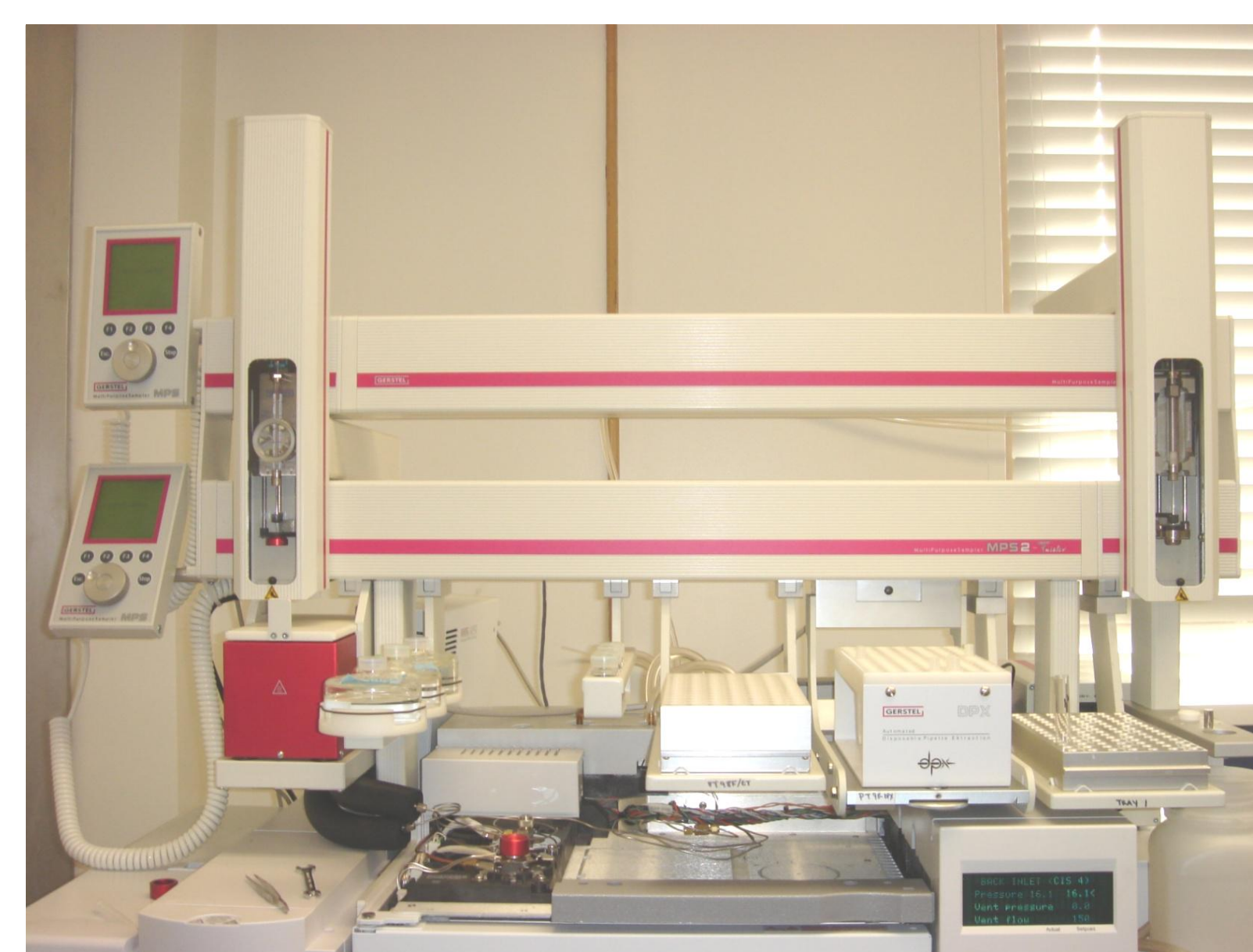
Figure 2. Dual rail MPS system on top of the GC/MS instrument for “just in time sample preparation” using automated QuEChERS tips.
