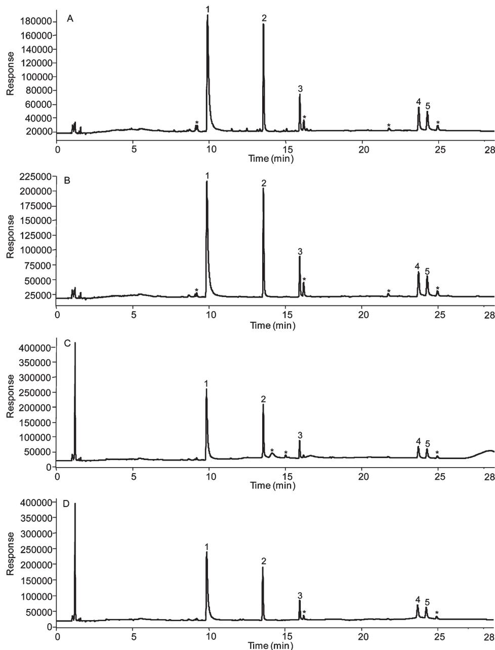
**Figure 4.** Representative GC-ECD chromatograms of DPX extracted 0.5 ppm bifenthrin, captan, chlorothalonil, and esfenvalerate in (A) yellow squash, (B) tomato, (C) carrot, and (D) tangerine. Separation was performed using a DB-17 column. Peak identification: 1, chlorothalonil; 2, captan; 3, bifenthrin; 4, esfenvalerate 1; 5, esfenvalerate 2. Peaks marked with an asterisk (\*) are matrix derived.
