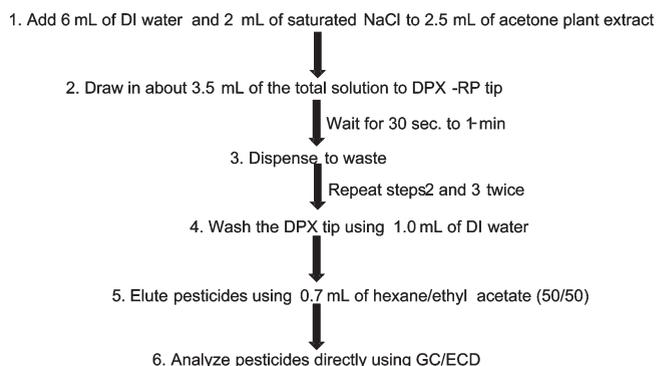
**Figure 2.** Schematic flow diagram of the DPX method for extraction of multiresidue pesticides in fruits and vegetables for GC-ECD analysis (method 2).
