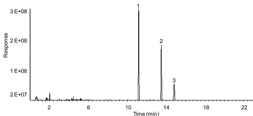
**Figure 6.** GC-ECD chromatograms of DPX extracted from tomatoes from produce. Separation was performed using a DB-608 column. Pesticides identified correspond to (peak 1) endosulfan I, (peak 2) endosulfan II, and (peak 3) endosulfan sulfate and bifenthrin.
