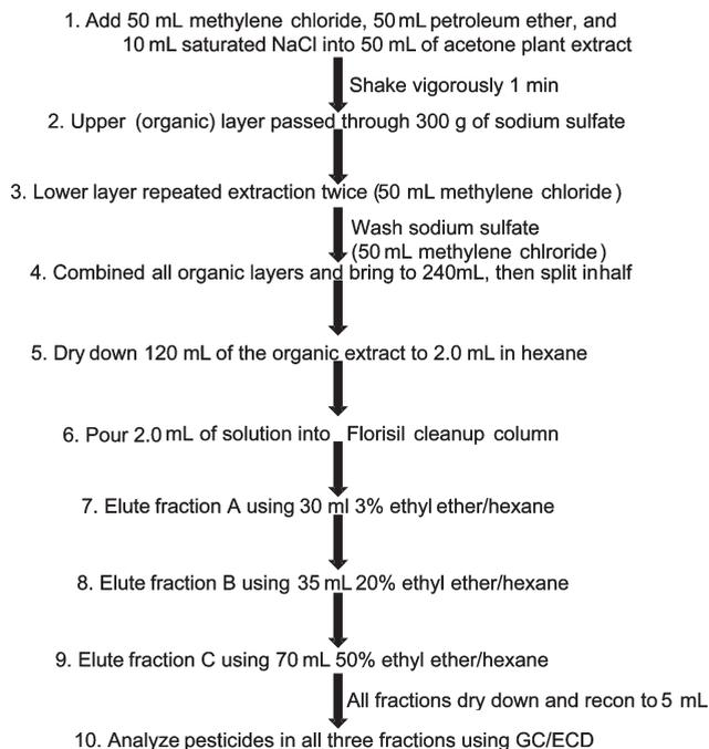
**Figure 1.** Schematic flow diagram of modified Luke method for extraction of multiresidue pesticides in fruits and vegetables for GC-ECD analysis (part of method 1). For analysis of OP pesticides, the other half of the 240 mL (120 mL) in step 4 is solvent evaporated and concentrated for direct analysis using GC-NPD.
