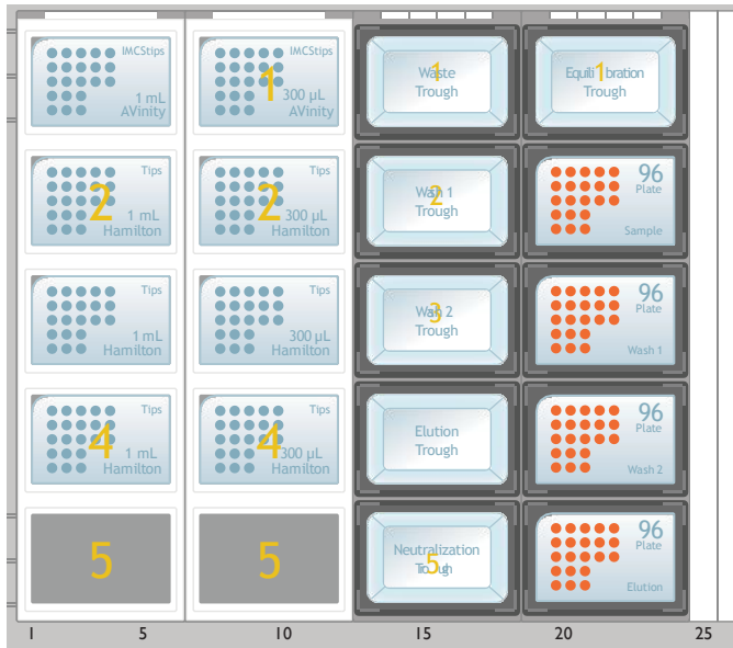
Figure 1. Typical deck layout for affinity purification followed by buffer exchange.
